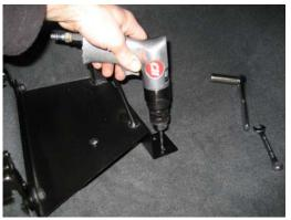
Pre-drill floor of vehicle with 3/16" drill bit Use holes in the "Z" bracket as a drill template
